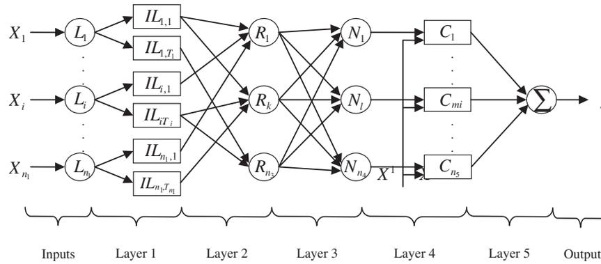
Fig. 4.2. Structure of the ANFIS network.
