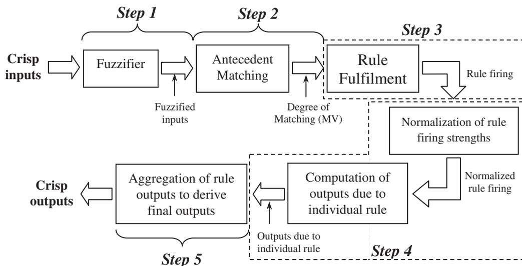
Fig. 4.1. Inference process of the TSK fuzzy model.
