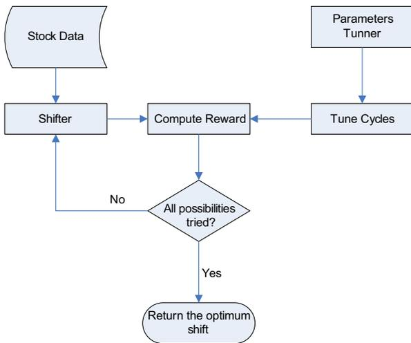
Fig. 3.11. Flow of the shift tuning algorithm.
