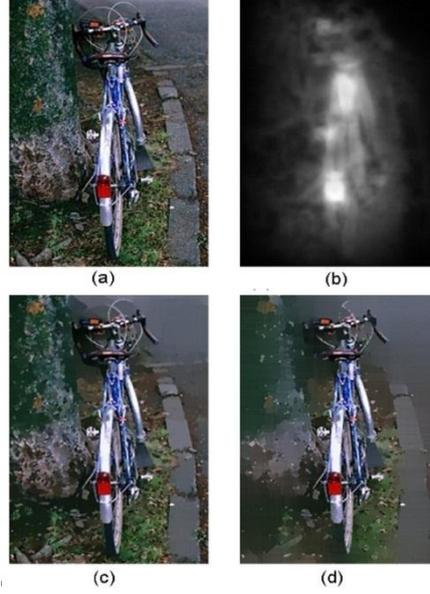
Figure 3. An example of comparison between non-linear diffusion and saliency driven nonlinear diffusion: (a) The original image; (b) Saliency map; (c) Nonlinear diffusion at scale 10; (d) Saliency driven nonlinear diffusion at scale 10.
