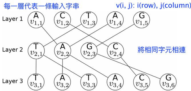
Fig. 1. The undirected multi-layered graph  $G$  obtained from the LCS instance ( $S = \{s_1 = \text{ACTAG}, s_2 = \text{TAGC}, s_3 = \text{ATACG}\}, \Sigma = \{A, C, T, G\}$ ).
