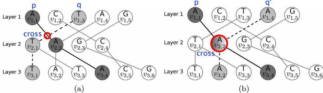
Fig. 2. Two examples of complete paths that cross, based on the LCS instance from Fig. 1. (a) Paths  $p = (1, 1, 2, 2, 3, 4)$  and  $q = (1, 3, 2, 1, 3, 1)$  cross because their corresponding edges between layers 1 and 2 cross. (b) Paths  $p = (1, 1, 2, 2, 3, 4)$  and  $q = (1, 4, 2, 2, 3, 2)$  cross because they both include vertex  $v_{2,2}$  from the second layer.
