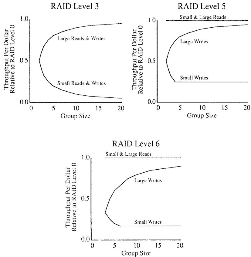
**Figure 6.** Throughput per dollar relative to RAID level 0. The graphs illustrate the tradeoff in performance/cost versus group size for each specified RAID level. Note that in this comparison, mirroring (RAID level 1) is the same as RAID level 5 with a group size of two.
