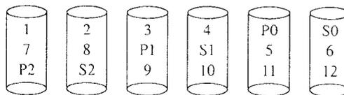
**Figure 9.** Distributed sparing. Distributed sparing distributes the capacity of the spare disk throughout the array. This allows all disks, including the disk that would otherwise have been a dedicated spare, to service requests. This figure illustrates a RAID level-5 disk array with distributed sparing. The 'P's denote parity blocks, and 'S's denote spare blocks.
