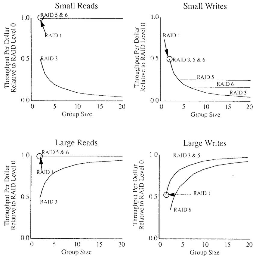
**Figure 5.** Throughput per dollar relative to RAID level 0. RAID level-1 performance is approximately equal to RAID level-5 performance with a group size of two. Note that for small writes, RAID levels 3, 5, and 6 are equally cost effective at small group sizes, but as group size increases, RAID levels 5 and 6 become better alternatives.
