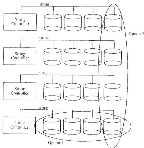
**Figure 7.** Orthogonal RAID. This figure presents two options of how to organize error correction groups in the presence of shared resources, such as a string controller. Option 1 groups four disks on the same string into an error correction group; Option 2 groups one disk from each string into a group. Option 2 is preferred over Option 1 because the failure of a string controller will only render one disk from each group inaccessible.
