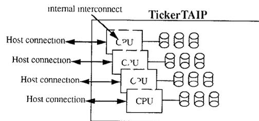
**Figure 12.** The TickerTAIP/DataMesh hardware architecture. A unique feature of the TickerTAIP architecture is the close association of a CPU to each disk drive in the array. This association allows each node to perform some of the processing needed to perform a disk array operation.
