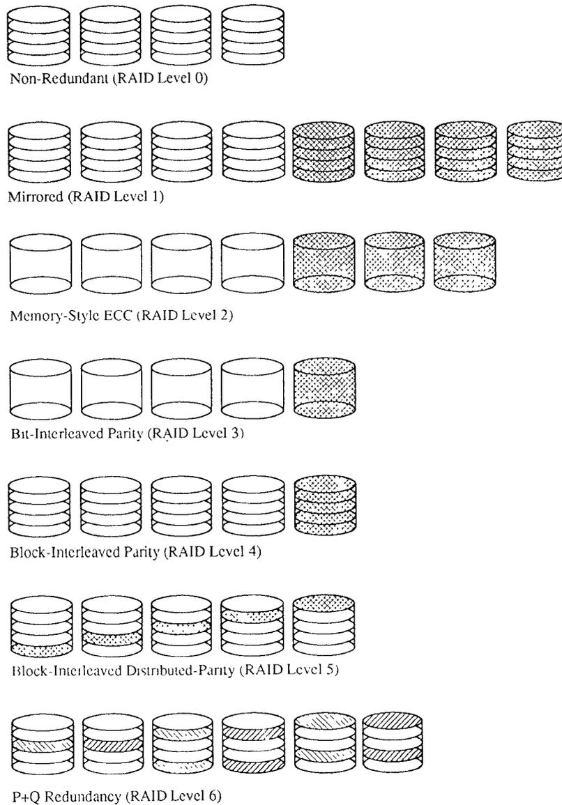
**Figure 3.** RAID levels 0 through 6. All RAID levels are illustrated at a user capacity of four disks. Disks with multiple platters indicate block-level striping while disks without multiple platters indicate bit-level striping. The shaded platters represent redundant information.
