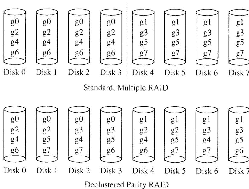
**Figure 8.** Standard versus declustered-parity RAID. This figure illustrates examples of standard and declustered-parity RAID with eight disks and a parity group size of four. Identically labeled blocks belong to the same parity group. In the standard RAID organization parity groups are composed of disks from one of two nonoverlapping subsets of disks. In the declustered-parity RAID, parity groups span many overlapping subsets of disks.
