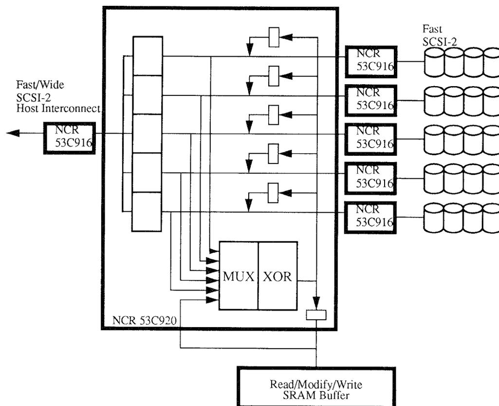
**Figure 11.** NCR 6298 controller data path. The lock-step data path of the 6298 requires no memory for any operations except RAID level-5 writes. By placing the XOR and MUX directly in the data path, the controller can generate parity or reconstruct data on the fly.
