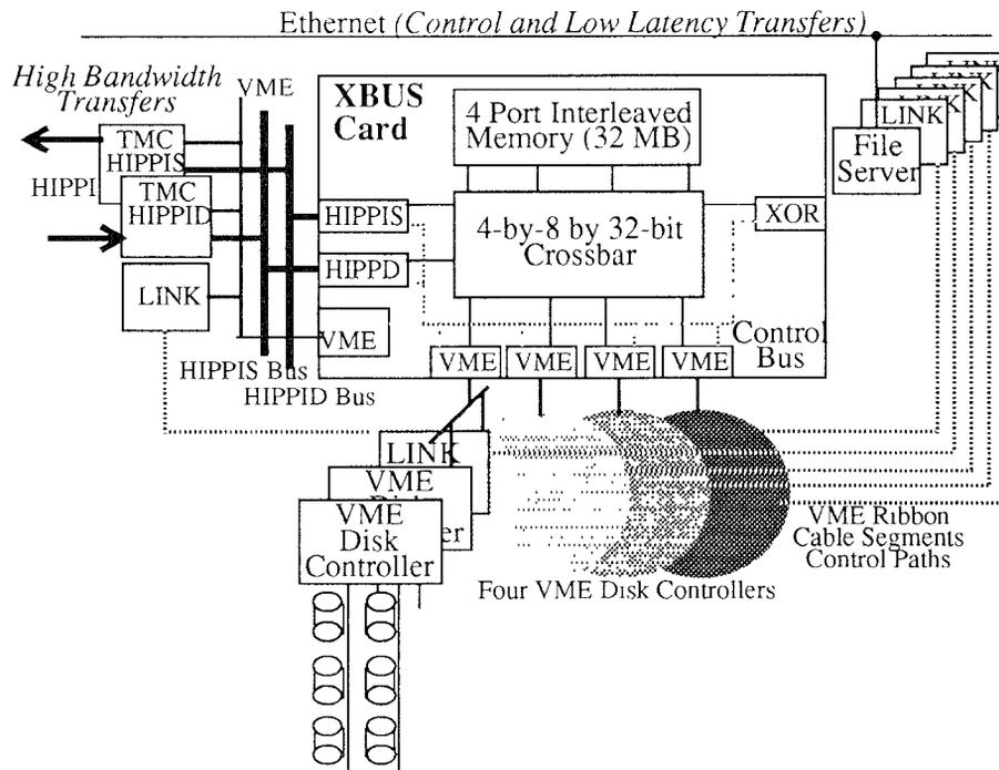
**Figure 13.** RAID-II architecture. A high-bandwidth crossbar connects the network interface (HIPPI), disk controllers, multiported memory system, and parity computation engine (XOR). An internal control bus provides access to the crossbar ports, while external point-to-point VME links provide control paths to the surrounding SCSI and HIPPI interface boards. Up to two VME disk controllers can be attached to each of the four VME interfaces.
