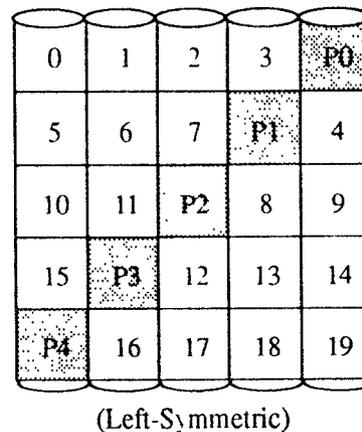
**Figure 4.** RAID level-5 left-symmetric parity placement. Each square corresponds to a stripe unit. Each column of squares corresponds to a disk. P0 computes the parity over stripe units 0, 1, 2, and 3; P1 computes parity over stripe units 4, 5, 6, and 7; etc. Lee and Katz [1991b] show that the left-symmetric parity distribution has the best performance. Only the minimum repeating pattern is shown.
