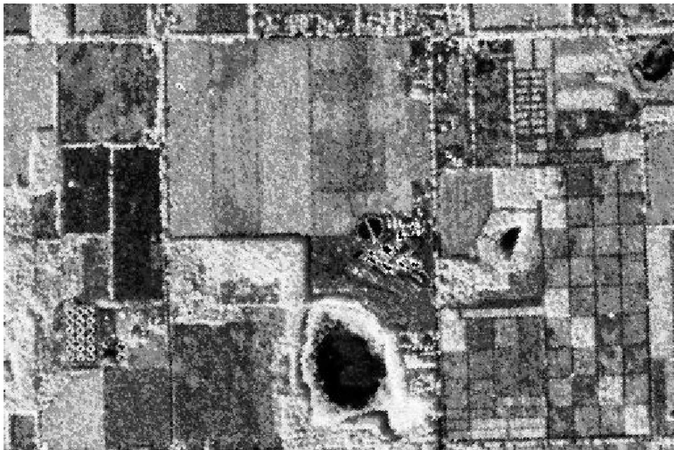
Fig. 2. SAR image of the test site at the Kellogg Biological Station. The square plots of homogeneous vegetation in the lower right of the image are 100 m on a side.
